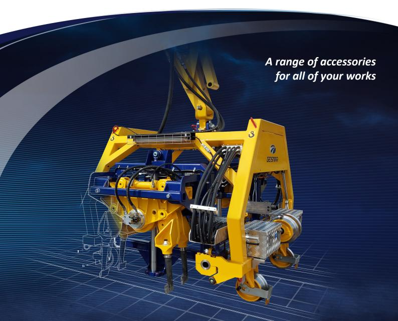
Tamping unit adaptable to multiple track configurations Remote-controlled operation and semi-automatic cycle Tamping quality and precision User-friendly operation and maintenance
